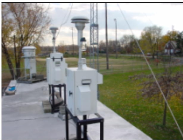
Figure 3: Manual Particulate Samplers located atop an Air Monitoring Trailer
